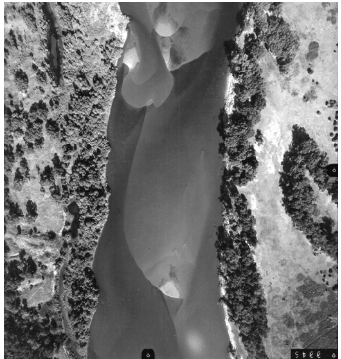
Figure 16. Sand sheets in bed of Feather River below the Feather-Bear confluence are composed largely of legacy sediment from the hydraulic-mining era. October 1998. (Source of photo: California Department of Water Resources.)
