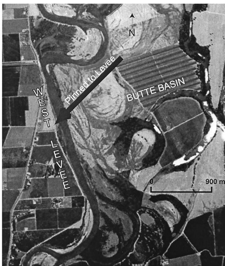
Figure 7. Aerial photograph showing main channel pinned to west levee (arrow) in reach 2. Levees on the west bank cut off the Sacramento River from Colusa Basin to the west and force overflow into Butte Basin to the east.
